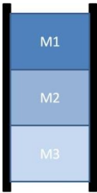
图 3 AMR 内部合金颗粒分布示意图 Fig.3 Schematic drawings of three-layered AMR
